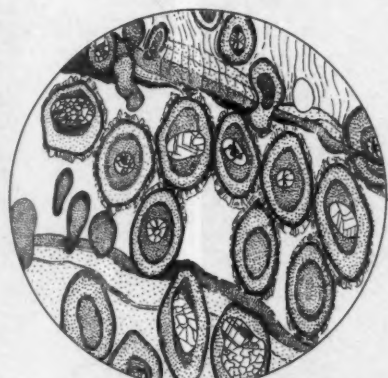
FIGURE 8. WELL-BEDDED OOLITE WITH ODD CENTERS AND GROWTH APRONS Cleavage begins to form (top). Conococheague limestone, Landis Creek between Hagerstown and Boonsboro. Spec. 271, ac section, deformation 30 per cent.
